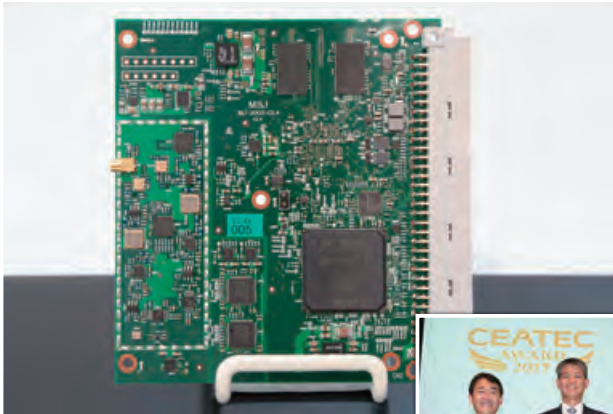
Next-Generation Multi-Frequency High-Accuracy Multi-Constellation GNSS Receiver Magellan Systems Japan, Inc.
